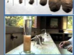
1. Fine aggregate containing more than allowable percentage of silt shall be washed so as to bring the silt content within allowable limits. 2. On the basis of particle size, fine aggregate is graded into four zones. 3. The volume increase of fine aggregate due to presence of moisture content is known as bulking.
