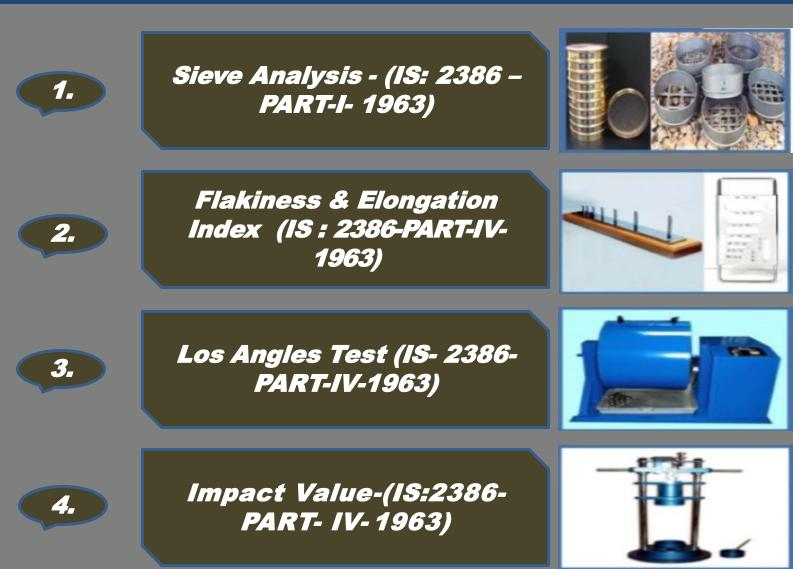
1. For Determination of the particle size distribution of Fine Aggregate and coarse aggregate. 2. For determination of the flakiness index and elongation index of coarse aggregate. 3. The Los Angeles (L.A.) abrasion test isa common test method used to indicate aggregate toughness and abrasion characteristics 4. For determination of the aggregate impact value of coarse aggregate, whichpasses <u>12.5 mm. IS</u> sieve and retained on 10 mm. IS sieve.
