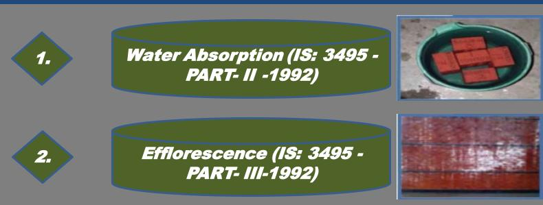
1. To determine the water absorption of bricks material. 2. To determine the qualify of bricks and salts affects on bricks.
